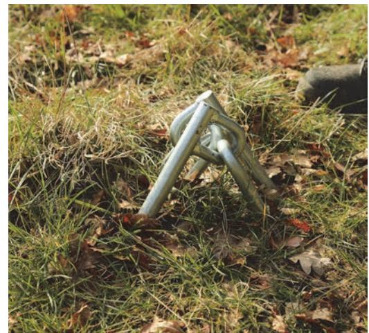
**5. Interlock the Moving Chain Links:** Jiggle the free chain links at the top of both Skewers so they are in a position to interlock, one sideways through the other.
